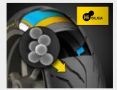
What is it? Compound blend combining wet grip resin in the shoulder compound with a very high silica ratio
