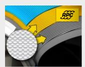
What is it? Front tyre carcass incorporating Rayon as ply material because of its thermodynamic properties
