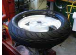
Fig. 3: Installing the second bead.
