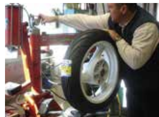
Fig. 5: Position uninflated tire vertically.
