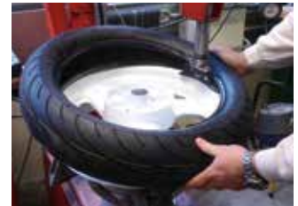
Fig. 2: Installing the first bead.
