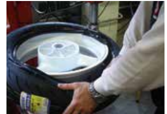
Fig. 4: Applying pressure to avoid stretching.
