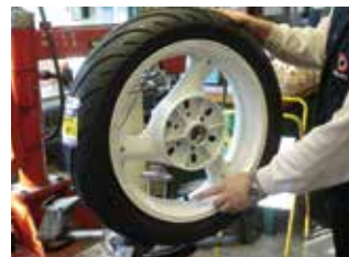
Fig. 5: Position uninflated tire vertically.
