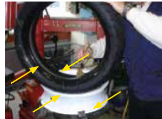
Fig. 1: Lubricating the tire and rim.
